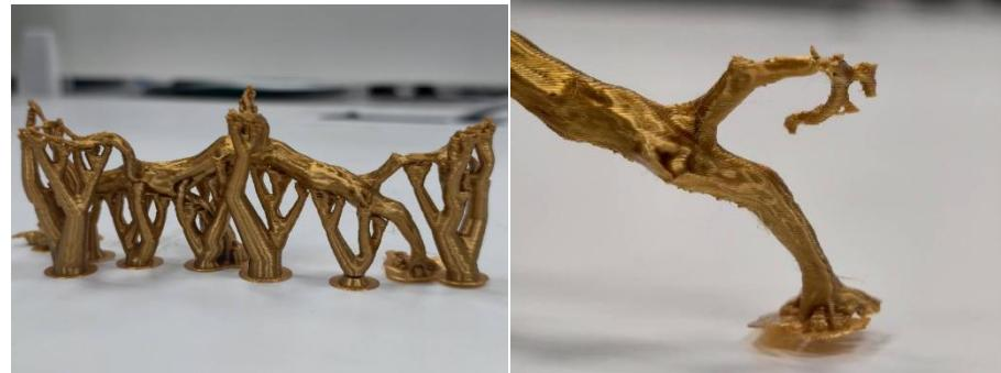
In such case, slightly increase the [Top Z distance] (e.g., from 0.2mm to 0.24mm/0.28mm) and reduce the [Branch Density] (e.g., from 30% to 15-20%). This reduces adhesion between support and model, lowering the chance of damaging the model during support removal.
